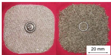
Textile electrodes with white PES non-woven, PU coating & press fastener pin on the outer side (left) & moss-embroidered terry-like inner side (right)
